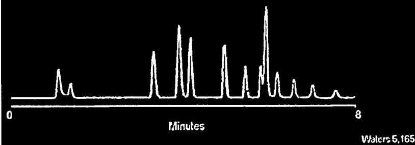
Figure 5 A rapid gradient separation with a 12-component test mix illustrates typical system reproducibility for gradient analysis. In this study of eight consecutive injections, the SDs for retention time were all less than 1 sec. Conditions—mobile phase: 5–95% B in 5 min, A = 0.1% aqueous formic acid and B = 0.07% formic acid in MeCN; flow rate: 10 \mu L/min; detection: 254 nm; column: Symmetry C 18 , 0.32 \times 150 mm; sample: 12-component small-molecule test mix.
